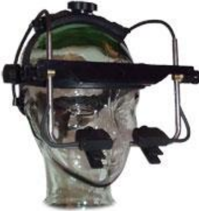
Figure 1.3: Eyelink II pupil eye-tracking system. Both right and left pupils are monitored with individual cameras. Accuracy of down to 30 arcminutes is expected, with the new Eyelink 1000 system having an accuracy of down to 15 arcminutes. http://www.sr-research.com/eyelinkII.html
