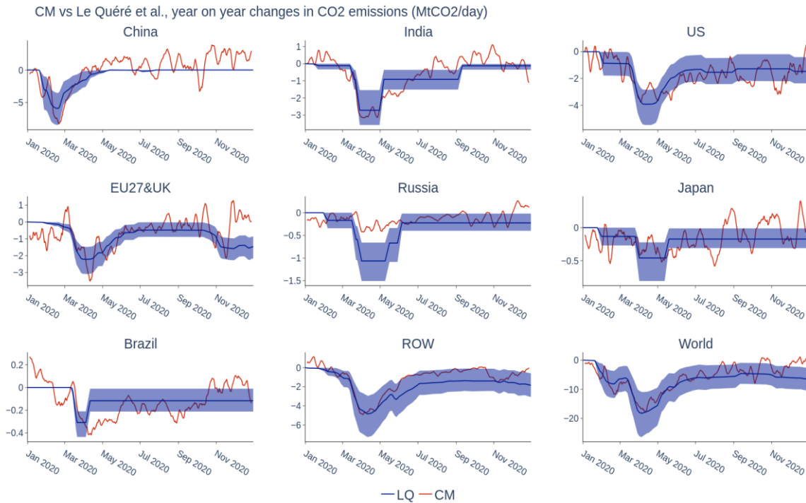
Fig 5: Comparison of year on year emission changes (2020 minus 2019) between Carbon Monitor (this study) and LQ by country. The Carbon Monitor daily data were applied a 7-days smoothing filter
