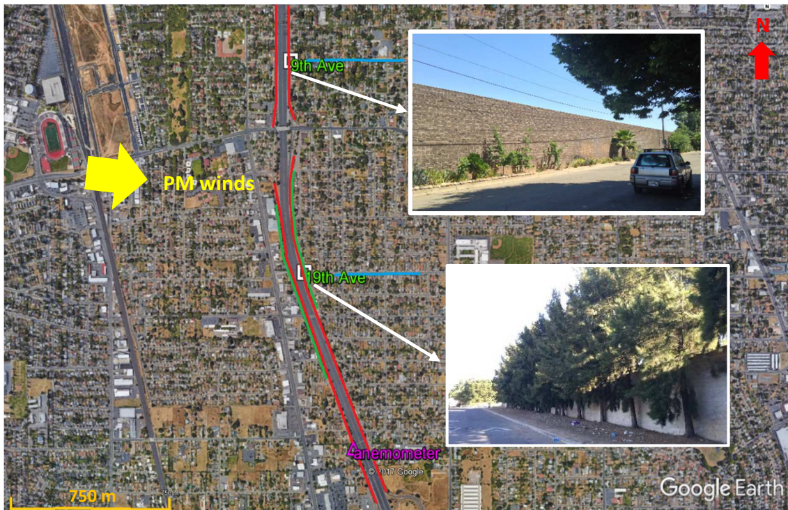
Fig. 12 The mobile sampling route at the SR-99 site in Sacramento, CA (blue lines). The green lines denote the vegetation barriers and the red lines denote the sound walls. Map source: Google Earth.
