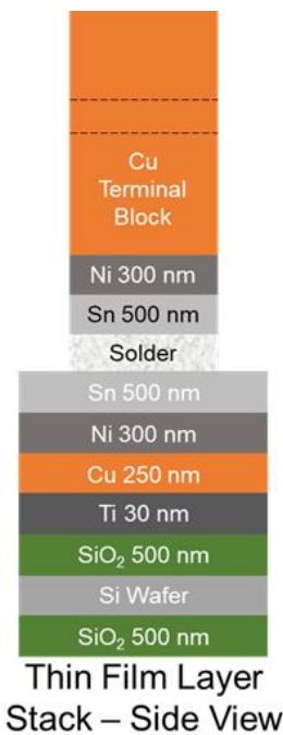
Figure 37: Attachment of copper block to silicon die is enabled through Ni and Sn thin films.
