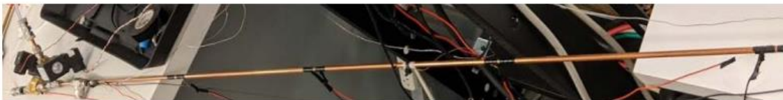
Figure 15: Horizontal tube setup for pressure wave propagation experiments, reproduced from [18].
