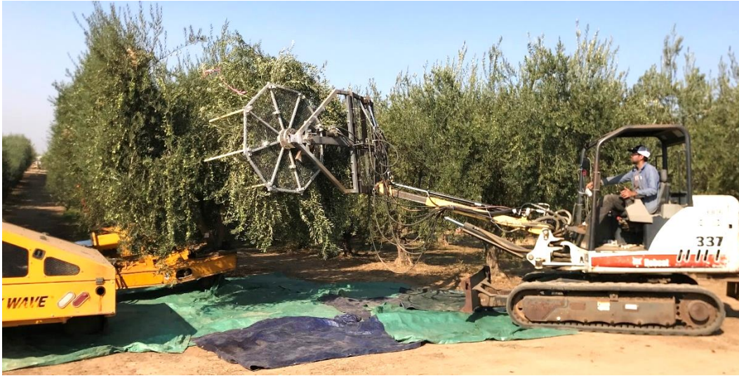
Figure 5.3 Trunk shaker and canopy shaker, shaking an olive tree simultaneously
