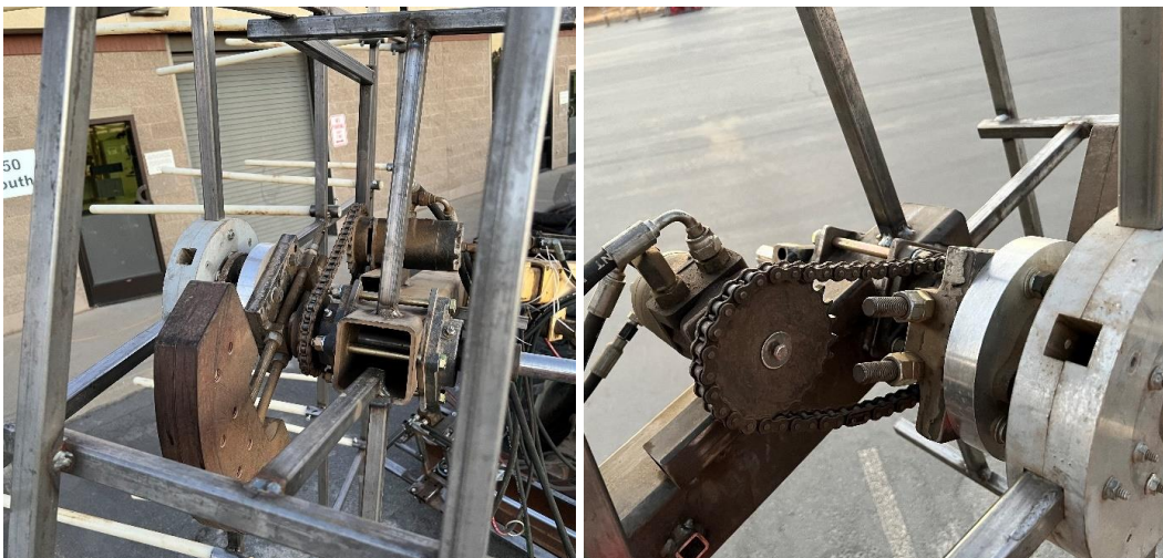
Figure.6.5 Internal mechanism used to generate circular oscillation movement in the canopy shaker.
