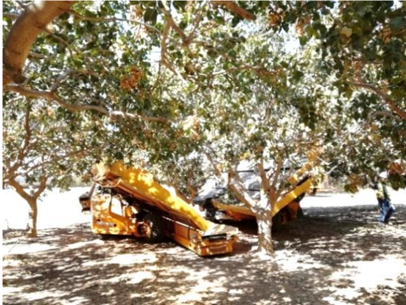
Figure 2.1 The C7 R-SERIES MK2 catching frame shaker by Custom Orchard Equipment was used in this experiment on a pistachio tree
