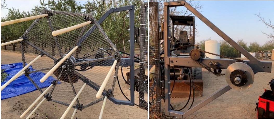
Figure 4.9 Modified design without shaking wheel attached (right) and with shaking wheel and rods attached (left)
