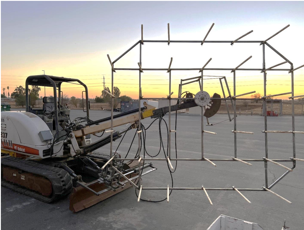
Figure.6.4 Newly designed canopy shaker built for old large olive trees in California.
