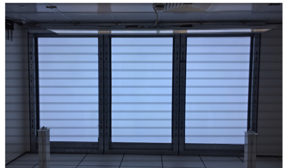
Fig. 13. Blinds open for \|Y_p(t) - Y_m(t)\|_\infty \geq 2000 .
