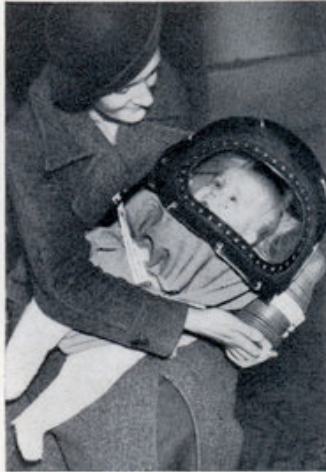
Pure air is fed to this infants' gas mask by operating the bellows with the hands
