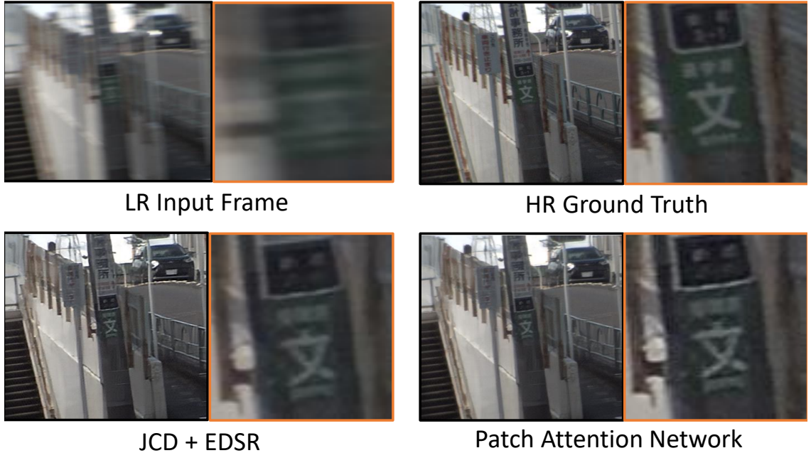
Figure 4.1: Patch Attention Network. We show frame on the left and zoomed in patch on the right. Top Left: Input LR rolling shutter frame (resized to HR frame resolution). Top Right: Global shutter ground truth HR frame. Bottom Left: Output of combination of state-of-the-art RSC method (JCD [127]) and SR method (EDSR [60]). Bottom Right: Predicted image by Patch Attention Network. It can be observed that the PatchNet model generates superior results as compared to state-of-the-art rolling shutter correction and super-resolution method.
