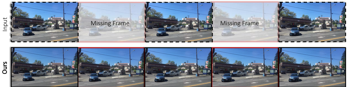
Figure 2.7: Representative video from Adobe240 dataset. The car at the bottom left has motion blur due to frame averaging as well as the motion of the car. Our proposed approach is able to enhance the frame by removing motion blur caused by frame averaging as well as object motion.
