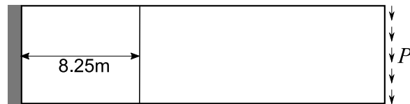
Figure 3.21: Cantilever Beam - Loads and Boundary Conditions
