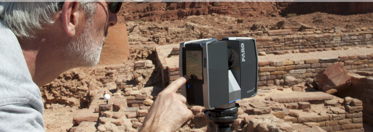
Collecting point cloud data with Faro laser scanner at Dedan, Saudi Arabia, for dissemination in 3D environments. Photograph by T. E. Levy, UC San Diego Levantine and Cyber-Archaeology Lab.
