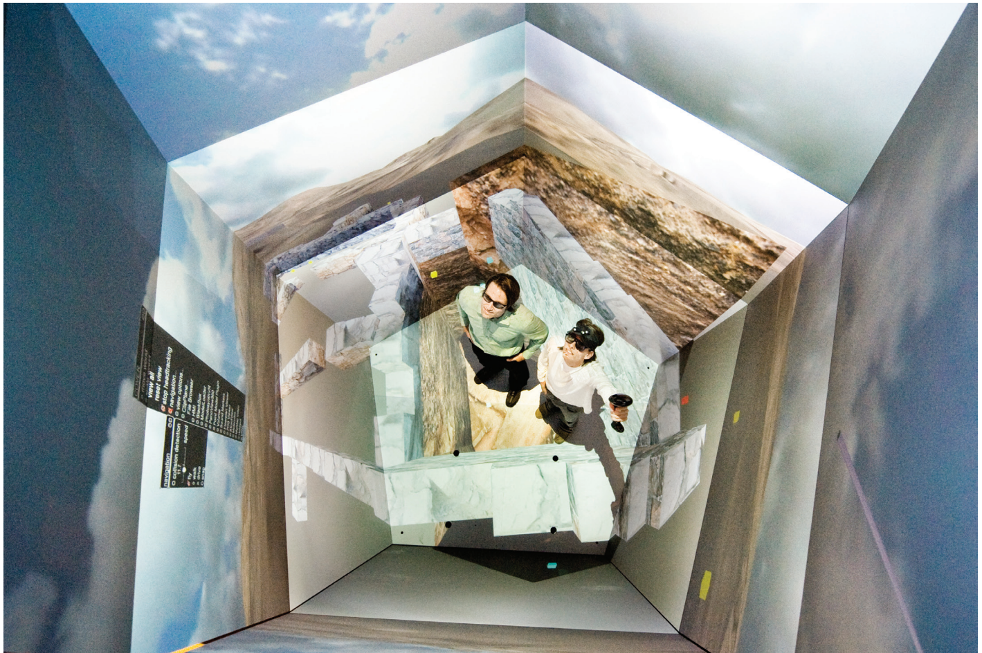
Figure 1. The StarCAVE at UC San Diego's Qualcomm Institute, showing the 360 degree, five-walled, fully immersive virtual reality system. This image shows the 3D model of the Iron Age copper smelting site Khirbat en-Nahas. Photograph courtesy Qualcomm Institute, UCSD.
