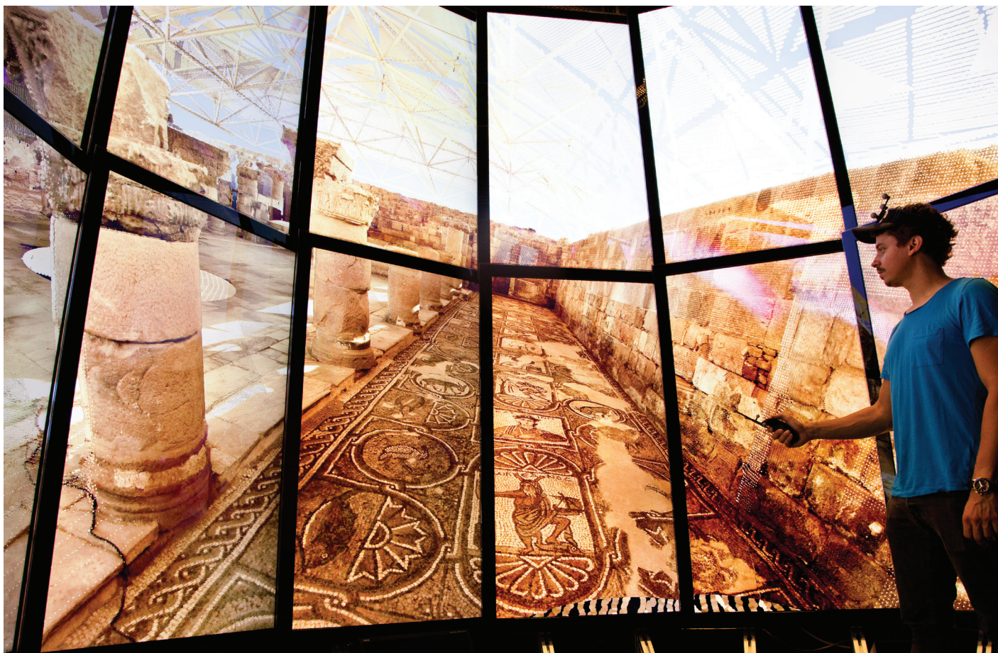
Figure 3 (below). The TourCAVE is a parabolic, semi-immersive virtual reality system. This image shows the mosaic floors of the Byzantine church at Petra in southern Jordan. Photographs courtesy Qualcomm Institute, UCSD.
