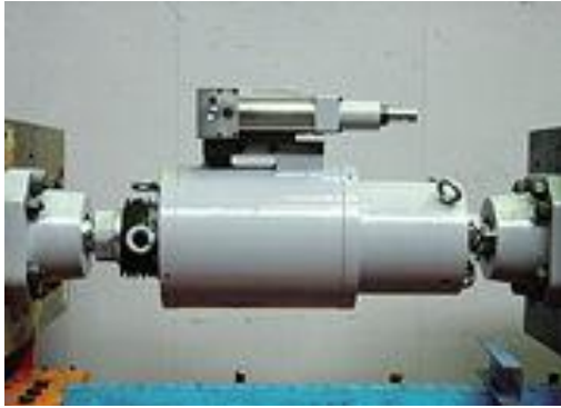
(a) HiDAXe Adjustable Passive Damper by Kajima
