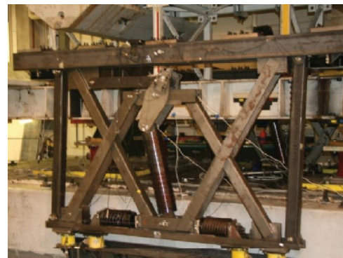
(b) Tested NSD frame undergoing a displacement input
