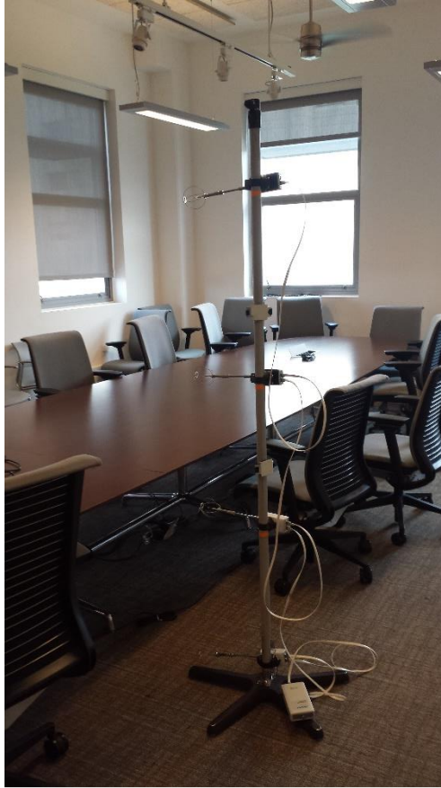
Figure 1: The anemometer tree replacing a chair at a conference table.
