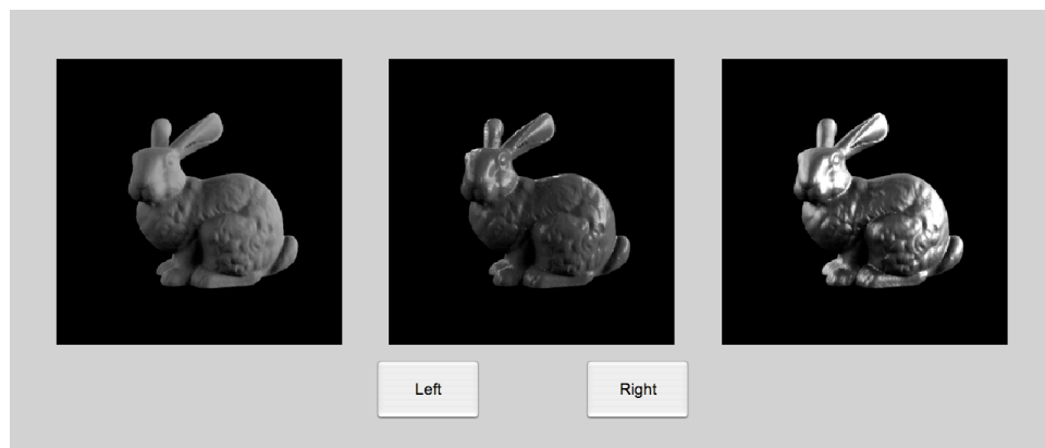
Figure 3.1 Screen capture from the distance comparison test. The subject is asked to click on the appropriate button to indicate which pair appears more similar, Left : Left + Middle, or Right : Middle + Right.
