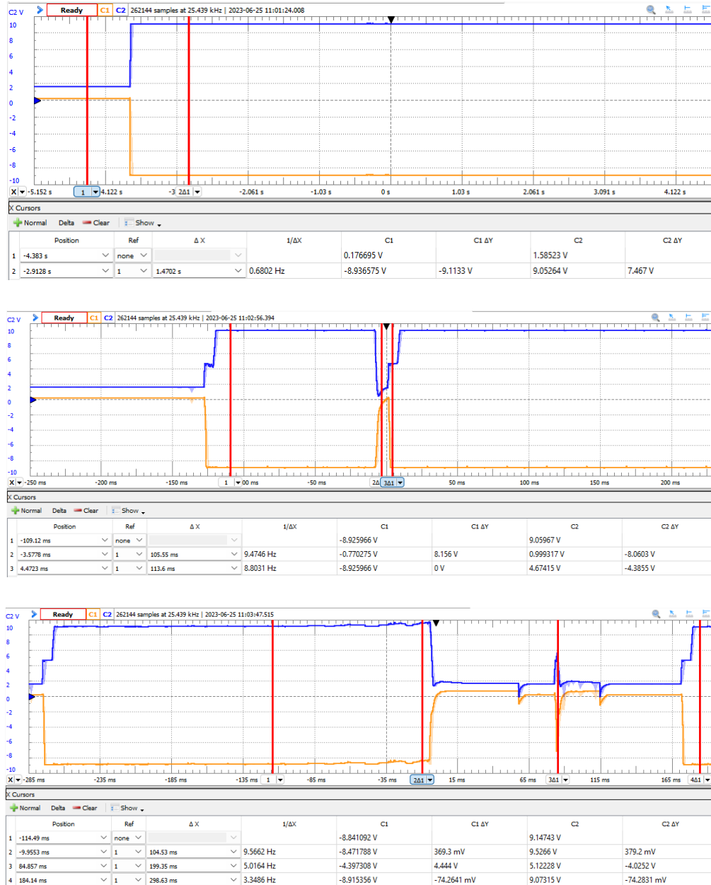
Figure A.7 9 V rails. Top, ideal +/-9 V supply rails. Middle, unexpected fluctuations in supply rails during operation. Bottom, power spiking on supply rails after disconnection and reconnection.
