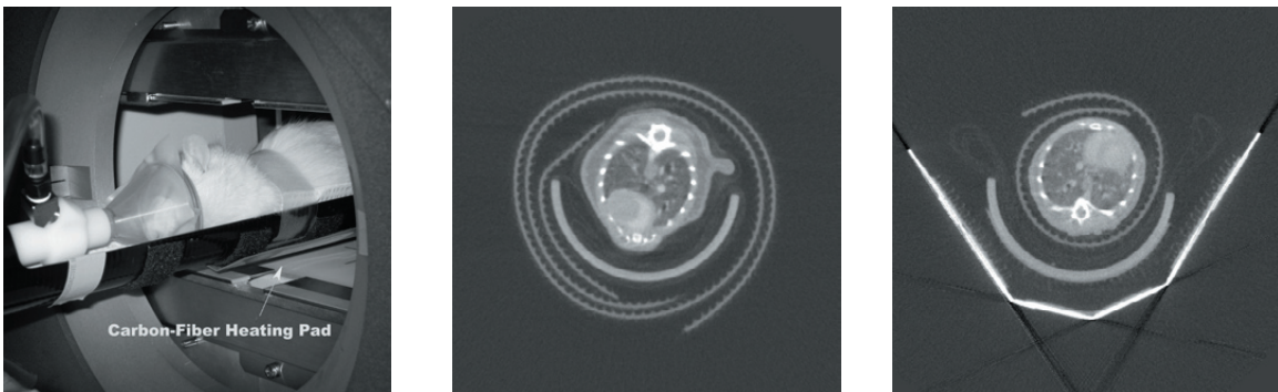
Figure 43: Carbon Fiber System Geometry During Imaging
