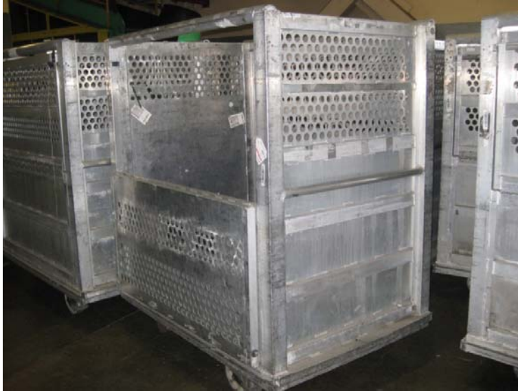
Figure 6-2. USPS Containers used by FedEx, small enough to fit in BART car
