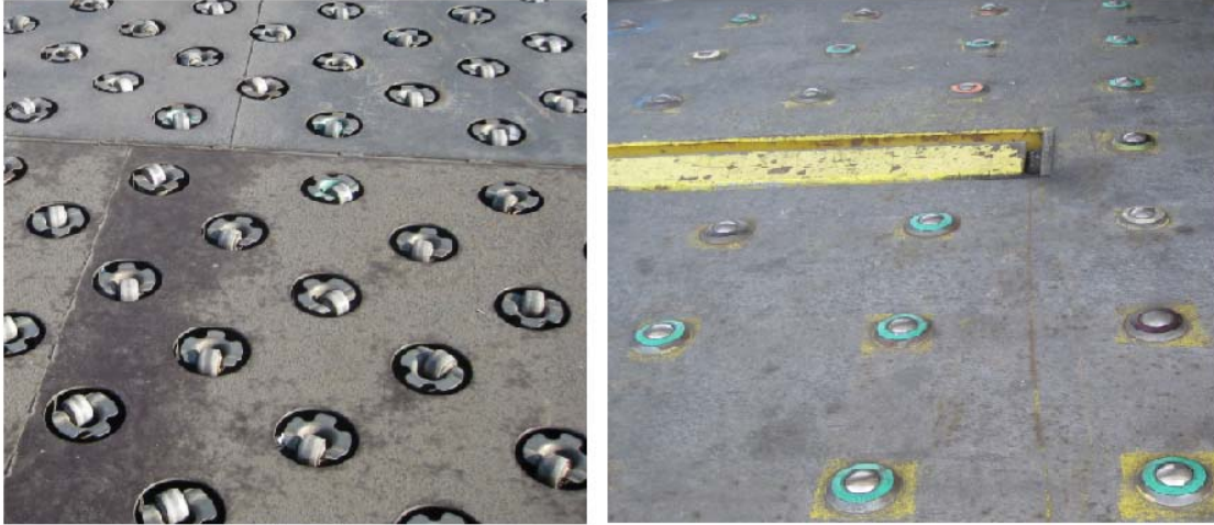
Figure 6-6. Roller Mat or Ball Bearing for Container Transshipment (Source: FedEx Western Regional Hub)
