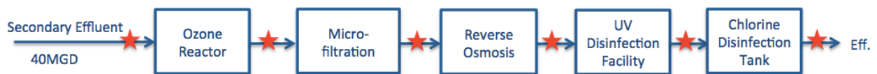
Fig. 3. Schematic of wastewater treatment processes at ECLWRF. Stars indicate sampling locations of this study.
