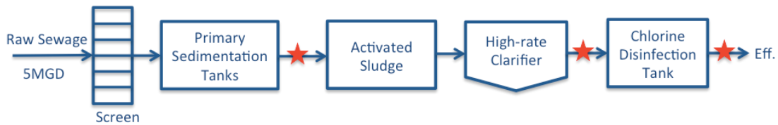
Fig. 2. Schematic of wastewater treatment processes at CWRP. Stars indicate sampling locations of this study.
