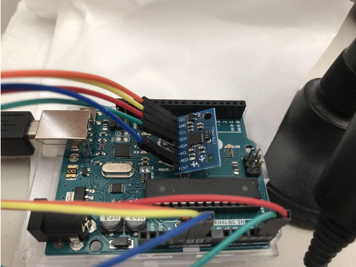
Figure 4.1: Arduino-Uno with MPU-6050 inertial sensor
