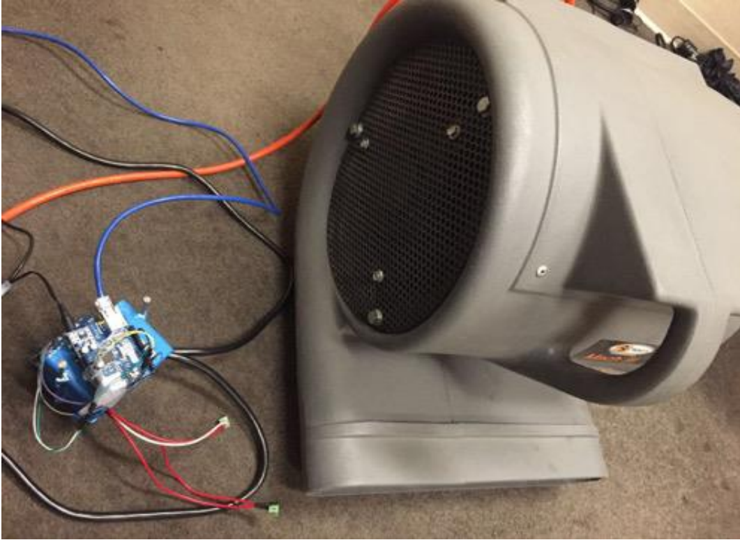
Figure 3.2c: Wind machine simulation with Arduino Ethernet Shield
