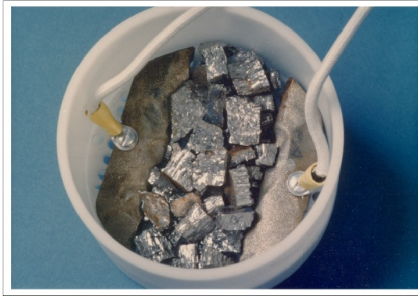
Figure 12. Bi-Sb-Te TE material charges (in a cell) for spark erosion process.
