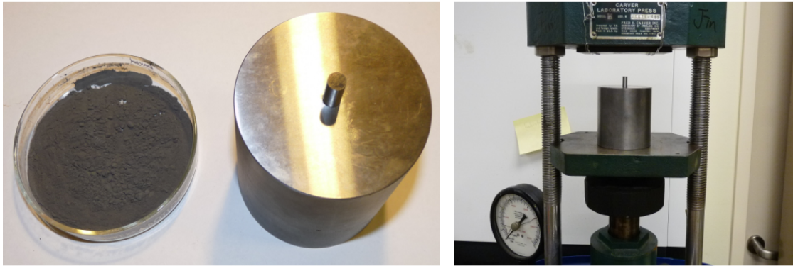
Figure 20. \text{Bi}_{0.5}\text{Sb}_{1.5}\text{Te}_{3.0} Powder and dies for pressing of TE powders with a force of up to 10,000 lbs.
