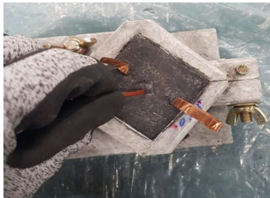
(f) Insertion of thermocouple
