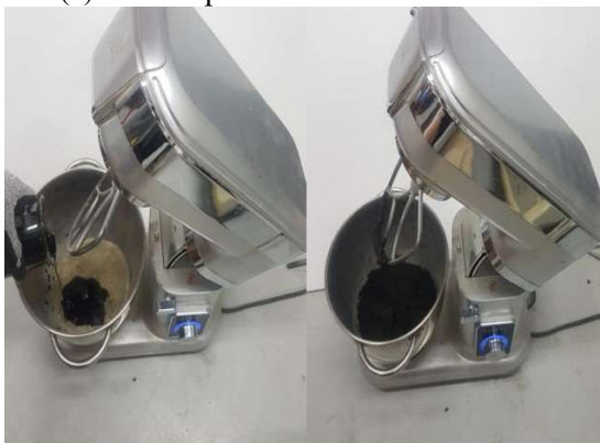
(c) Mixing of MWCNT dispersion (3 min)
