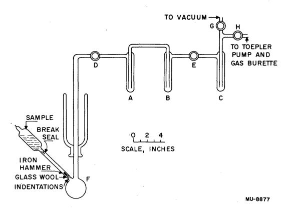
Fig. 2. Apparatus for recovering gases from liquids.
