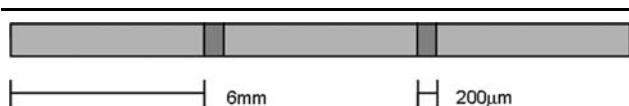
Fig. 1. Sample configuration. The cross-section is a square, approximately 400 \mu m × 400 \mu m.
