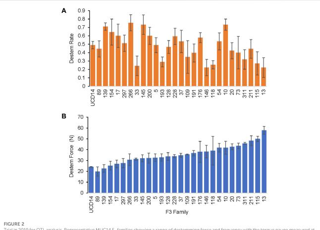
Trial in 2019 for QTL analysis. Representative MUC14 F<sub>3</sub> families showing a range of destemming force and frequency with the torque gauge measured at the mature green stage. (A) Mean fraction of fruits cleanly destemmed and (B) mean destemming force for each family. Error bars represent standard error of replications.
