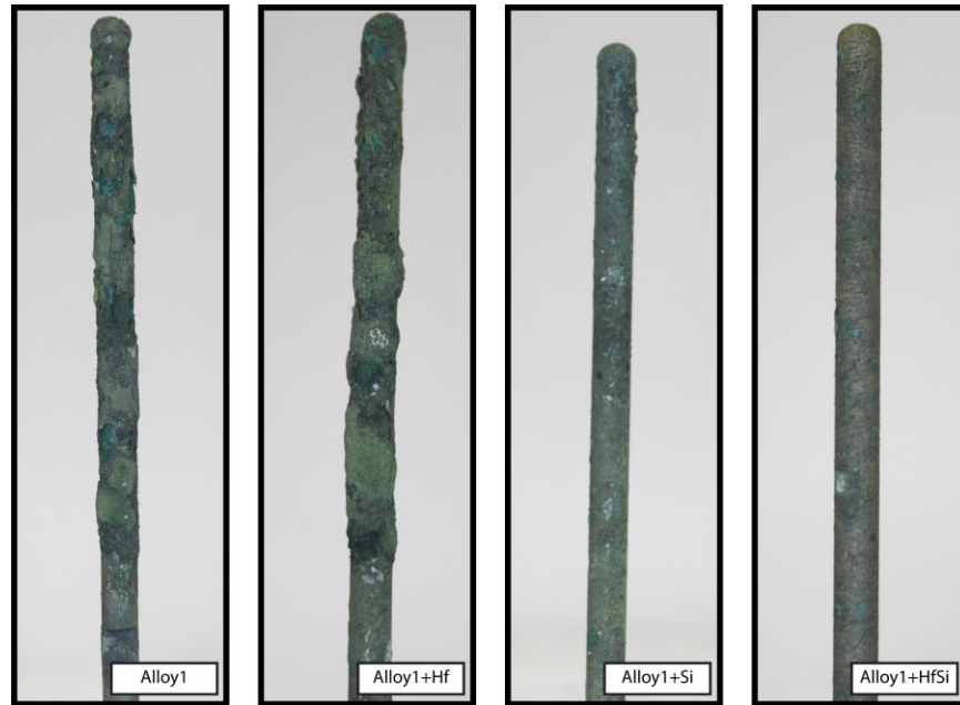
FIGURE 22. Image of Alloy1 and its doped variations post-exposure.
