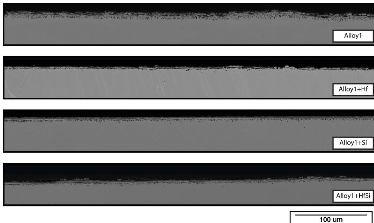
FIGURE 36. Backscattered SEM images of cross-sections of Alloy1 and its doped variations after pre-oxidation treatment PreOx1 followed by a 10-hour LVBR exposure.
