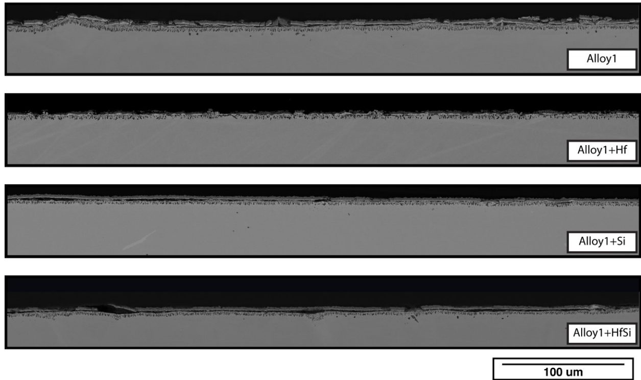
FIGURE 30. Backscattered SEM images of cross-sections of Alloy1 and its doped variations after a 10-hour LVBR exposure.
