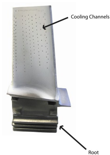
FIGURE 18. Image of a turbine blade where the root and cooling channels, both uncoated areas susceptible to hot corrosion attack, are highlighted [77].
