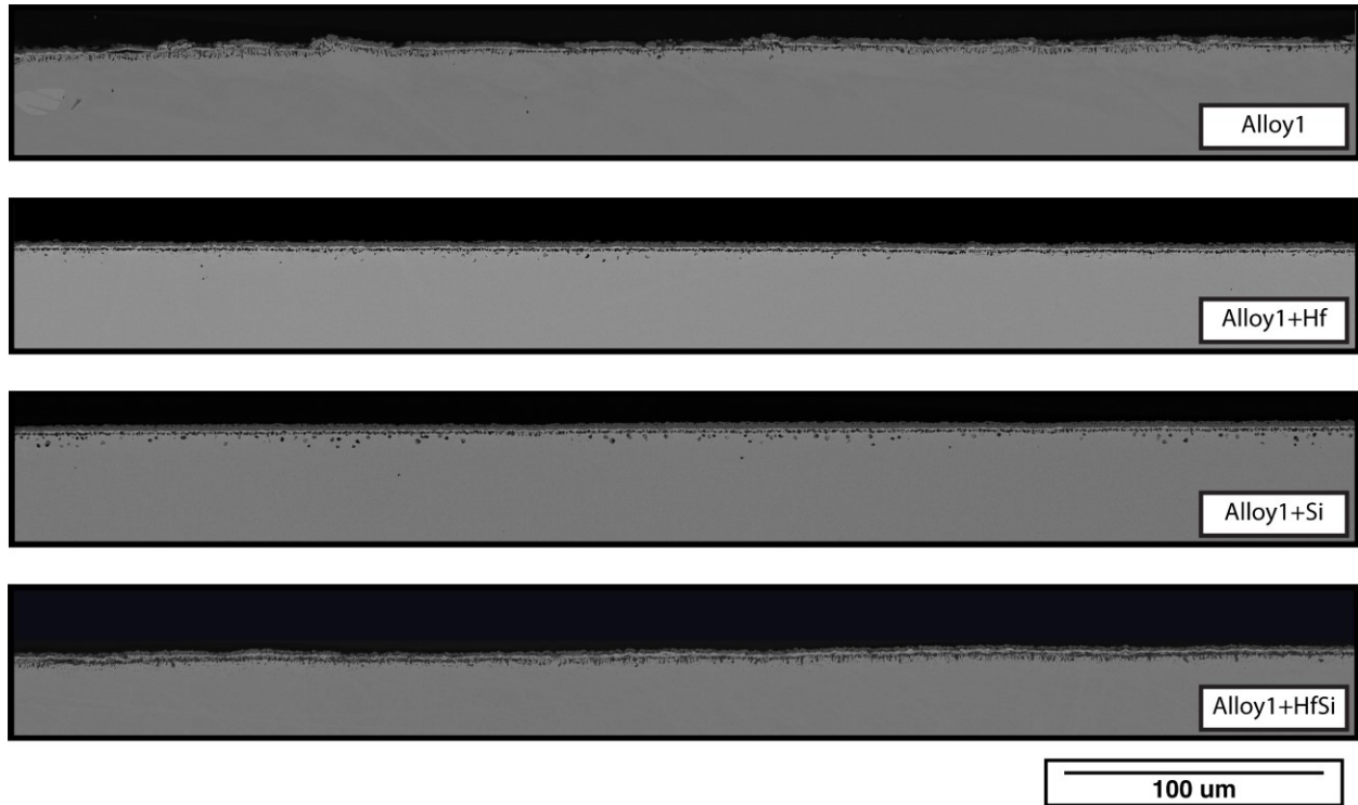
FIGURE 37. Backscattered SEM images of cross-sections of Alloy1 and its doped variations after pre-oxidation treatment PreOx2 followed by a 10-hour LVBR exposure.
