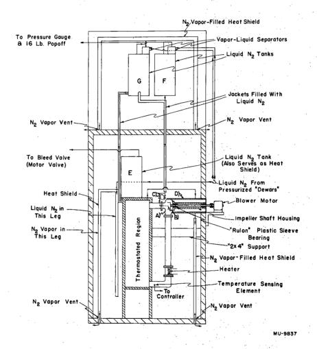
Fig. 6. Cold thermostat, elevation. A-Stainless steel centrifugal blower. B-Liquid nitrogen jet. C-Coarse and fine control valves for liquid nitrogen coolant. D-Access box for blower, impeller, bearing, etc. E-Liquid nitrogen tank confining cooling coil for high-pressure gas return. F-Liquid nitrogen "pressure" tank, provides liquid nitrogen for thermostat cooling. G-Liquid nitrogen "atmospheric" tank, provides liquid nitrogen for tank E.
