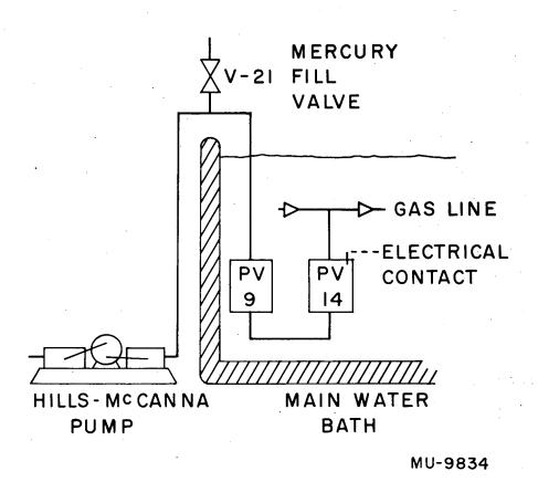
Fig. 4. Mercury piston pump.
