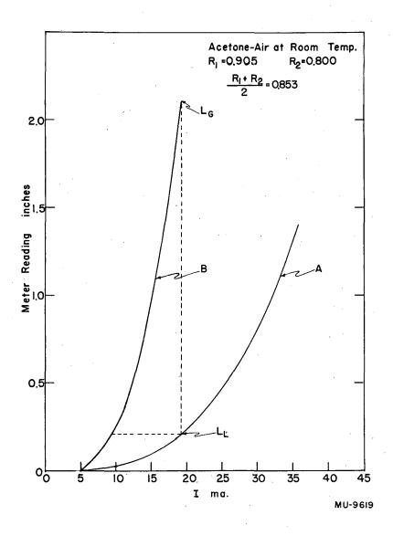
Fig. 22. Curve for calibration of liquid-level indicator, acetone-air at room temperature.
