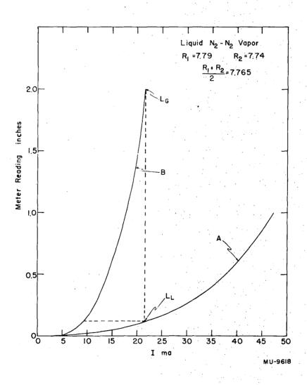
Fig. 23. Curve for calibration of liquid-level indicator, liquid nitrogen-nitrogen vapor at 1 atmosphere.
