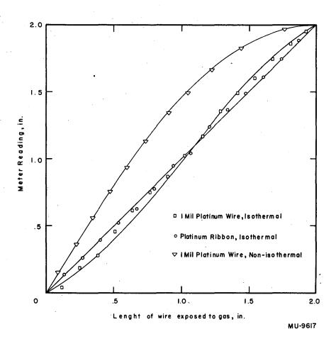
Fig. 24. Linearity of liquid-level indicator.
