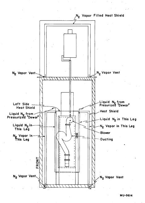
Fig. 5. Cold thermostat, side view.
