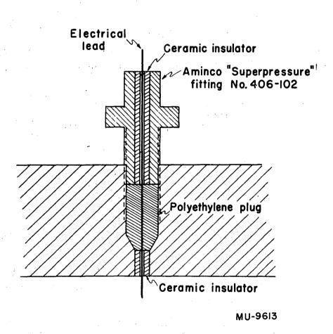
Fig. 17. Electrical connector for room-temperature operation.
