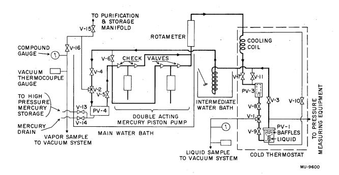
Fig. 1. Simplified flow diagram of recirculation equipment.
