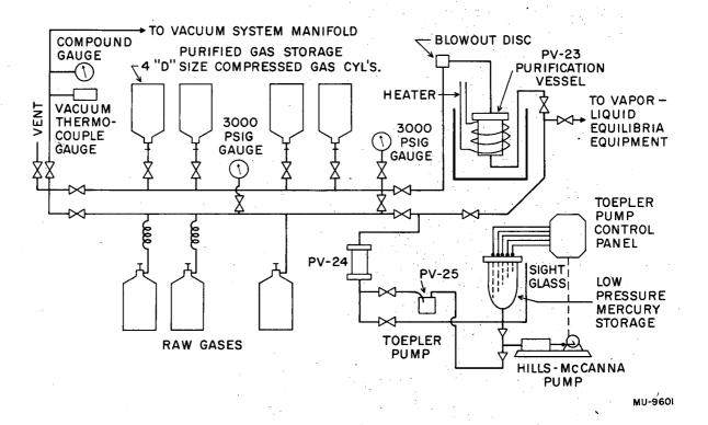
Fig. 14. Gas manifold and purification equipment.
