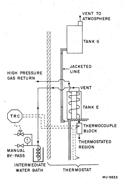
Fig. 9. Cooling of the return gas stream, early design.
