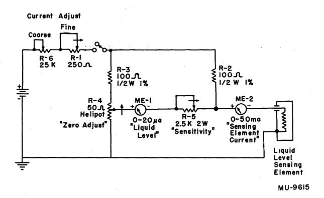
Fig. 21. Circuit diagram for liquid-level indicator.
