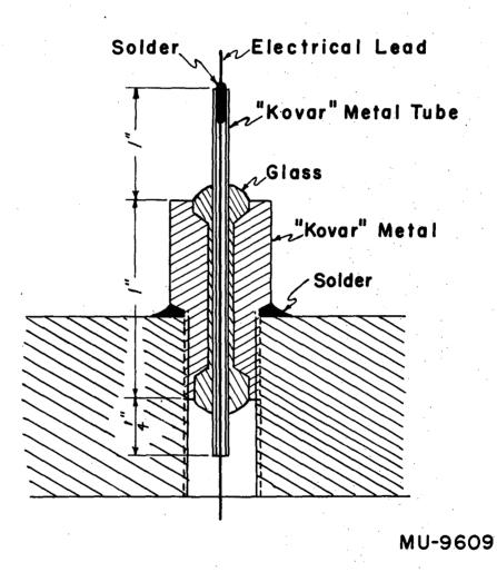
Fig. 18. Electrical connector for low-temperature operation.
