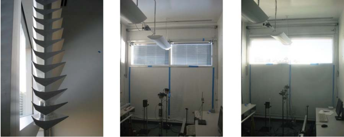
Fig. 2. Left: Side view of the OLS prior to being installed on the inward face of the clerestory glazing. The unit is then slid on the horizontal brackets at the top of the OLS and into the frame cavity. Middle: Interior view of the installed OLS. Right: Interior view of the installed Venetian blind reference condition.
