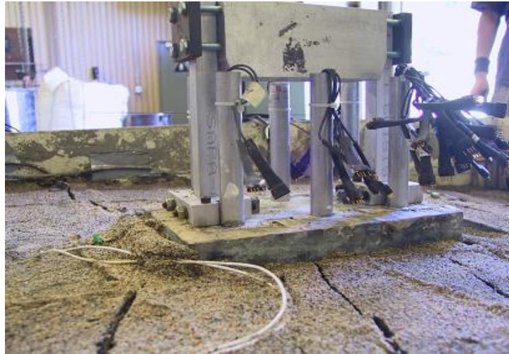
Fig 6: Photograph of pile cap after testing with the surficial layer of sand removed
