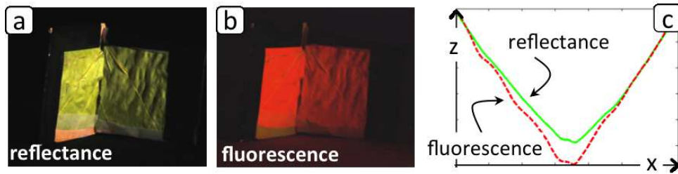
Figure 2.8: To demonstrate how fluorescence helps avoid mutual illumination, we covered a V-shaped cardboard with leaves. (a,b) The reflectance and the fluorescence images of the covered cardboard; (c) The shape was reconstructed using calibrated photometric stereo for both the reflectance and fluorescence channels. The reconstructed depth (at a certain cross section) is plotted for the reflectance and fluorescence images. While the reconstruction from the reflectance channel shows classical bending of the corner (pseudo surface) as described in [NIK90], the reconstruction from the fluorescence channel maintains sharp edges clearly demonstrating the reduction of the effect of inter-reflections.
