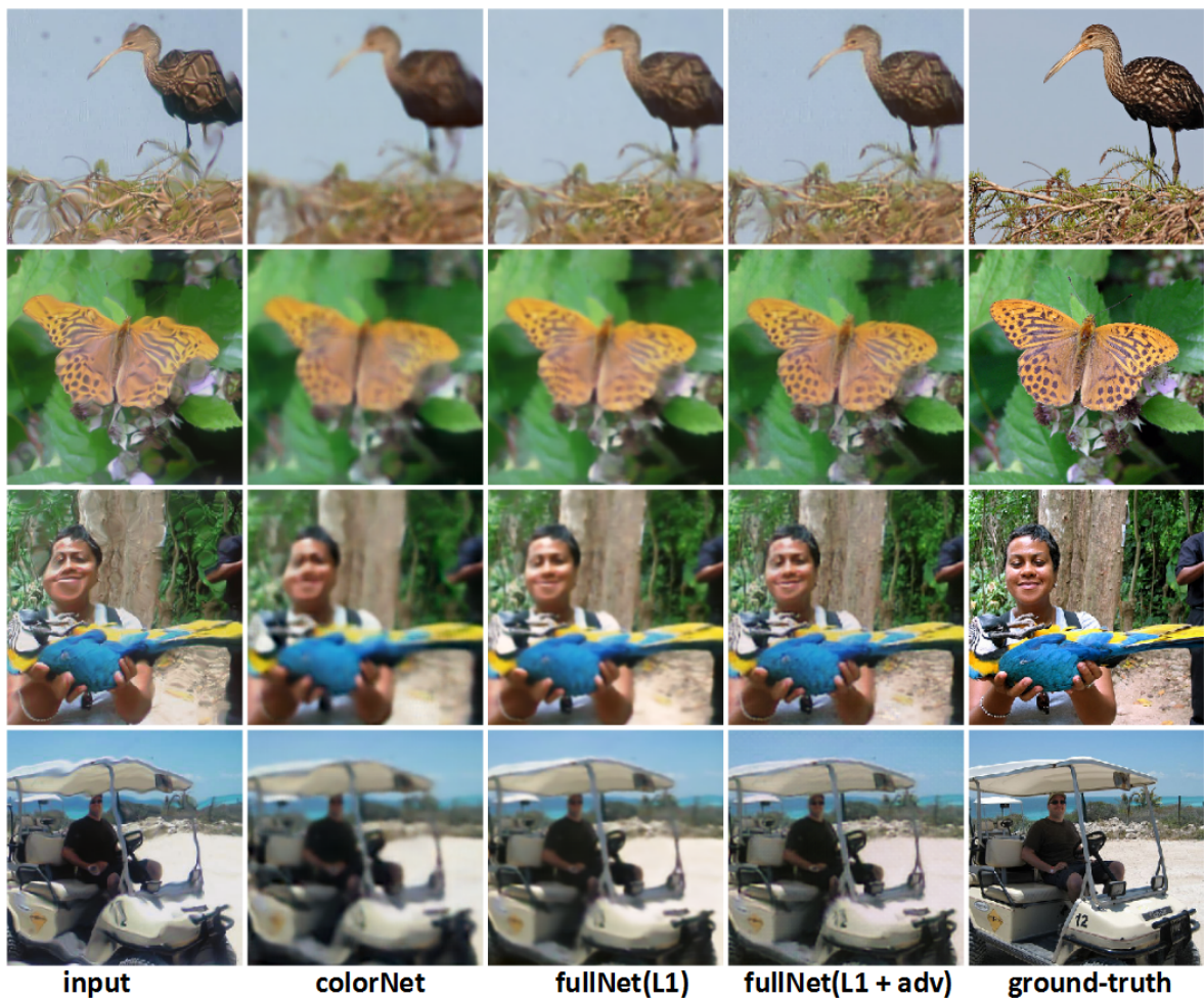
Figure 4.3: Qualitative results for ablation study on ImageNet validation test set. From left to right: input image, color net with L1 loss, warp+color net with L1 loss, warp+color net with L1+Adv+Per losses, ground truth. We observe that estimating the undistortion with the warp net significantly improves the geometry, while the adversarial loss allows better perceptual alignment to ground truth.
