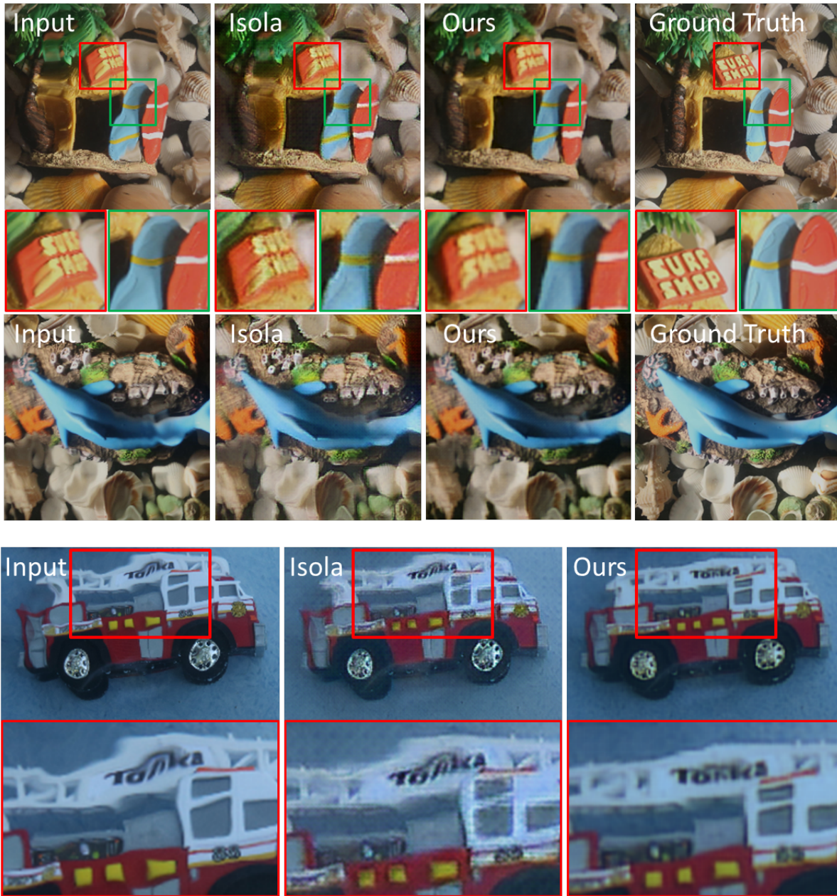
Figure 4.4: Results on real objects demonstrating generalization. (Rows 1 and 2) From left to right: input image in a larger tank, result of Isola et al. [IZZE16b], our result and ground truth. We observe that our framework that uses problem structure and careful normalizations produces better geometric undistortion and color outputs. (Bottom row) We show another example of further generalization by acquiring an image in a fountain pool. We see more significant contrasts relative to [IZZE16b], with clearly better undistortion performance for our method.
