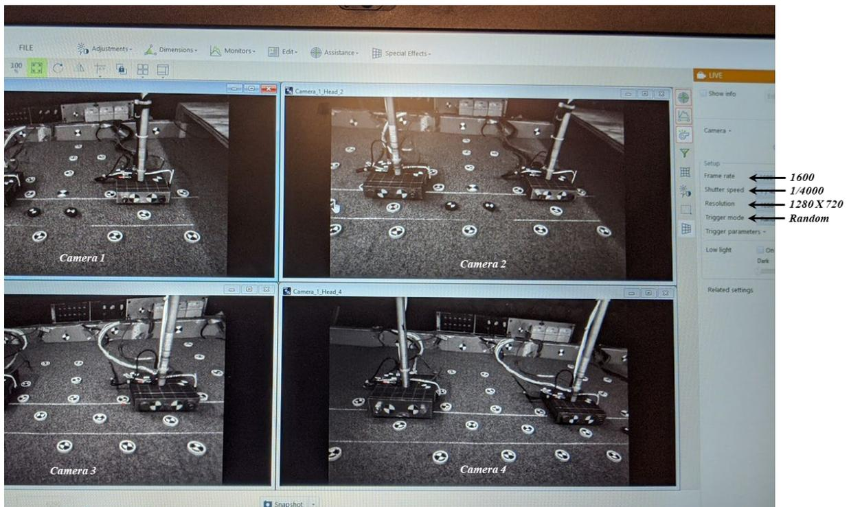
Figure 4.9. Live view of the model from the four Photron camera heads as viewed in the Photron FASTCAM Viewer.
