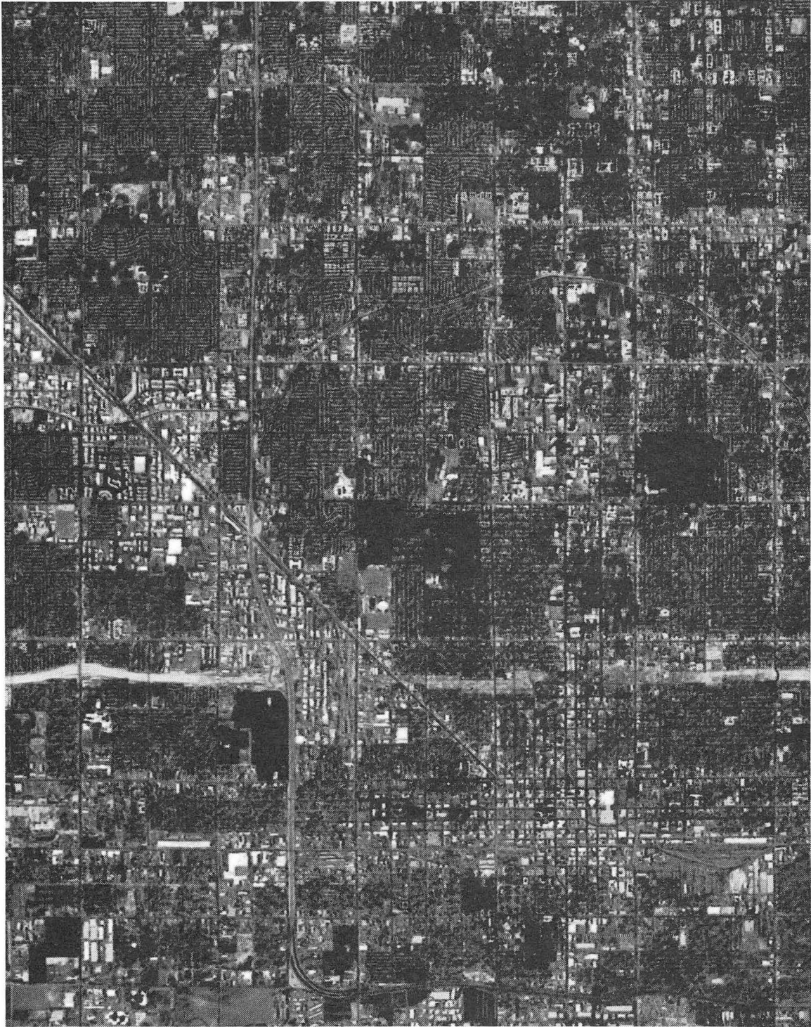
Figure 1. This black and white copy of a full color enhanced SPOT image of a segment of central Phoenix reveals only a part of the spatial information provided. Delimitation of urban terrain zones could easily be accomplished through photo interpretation of the original.
