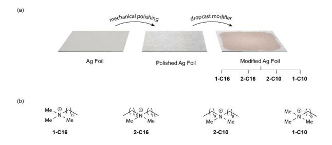
Scheme 1. Fabrication of modified Ag surfaces with quaternary ammonium salts. (a)
