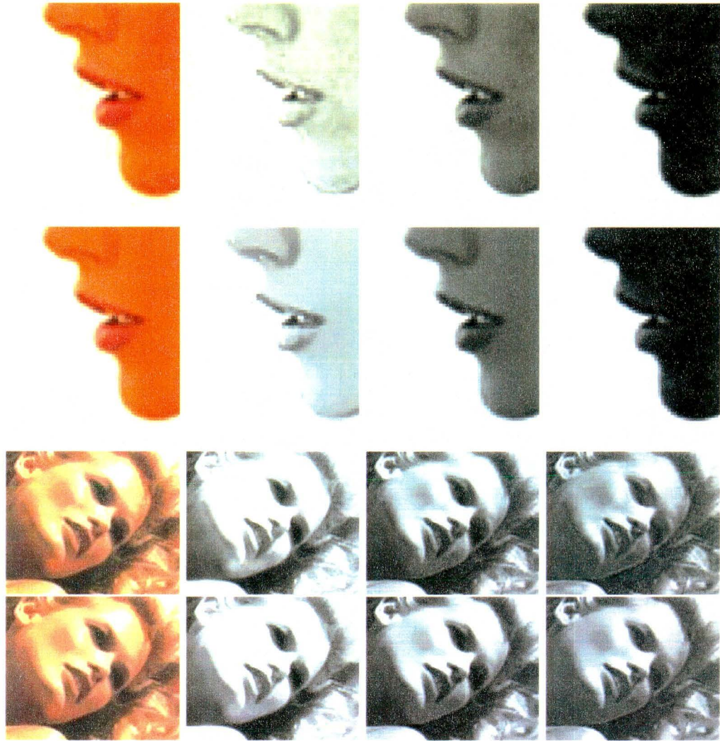
Figure 3: Denoising JPEG lossy compression perturbations. Rows 1&3: The original image and the three channels (R,G,B). Rows 2&4: The result of the Beltrami color flow (70 numerical iterations, \Delta t = 0.21 , \Delta x = 1 ). [This is a color figure]
