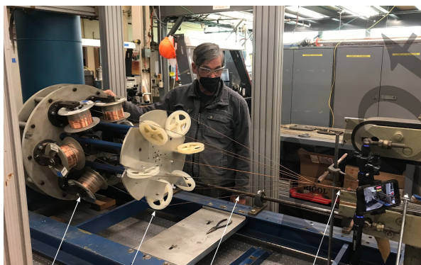
Figure 3. Hugh Higley and the cabling machine. A youtube video shows the cabling process.
