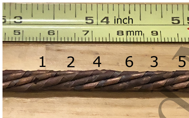
Figure 2. Cable 6a had a nominal diameter of 5.7 mm and a twist pitch length of 52 mm. Each STAR ® wire is also labeled.
