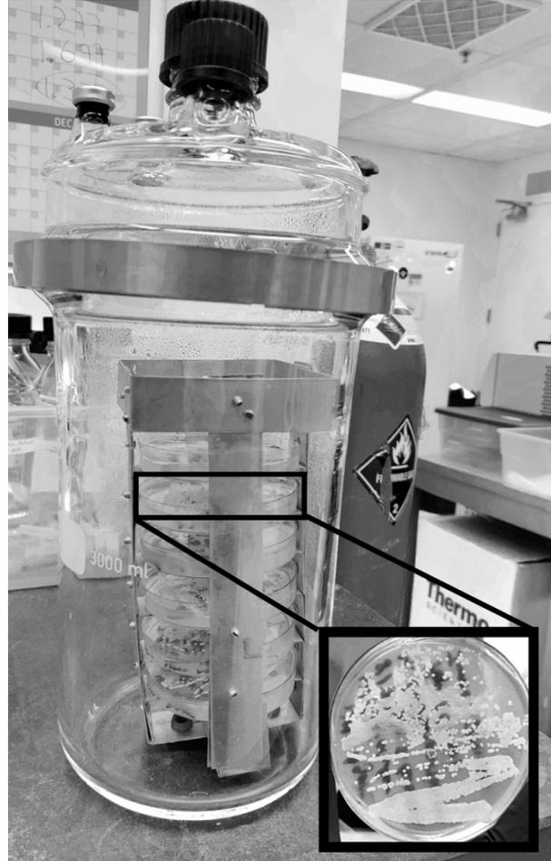
**Figure 4-1.** Three-liter glass flange flask containing *Methylosinus trichosporium* colonies on NMS agar plates. Agar plates are placed into shelves of a custom-built stainless-steel rack. Close up picture shows example of *M. trichosporium* colonies on an
