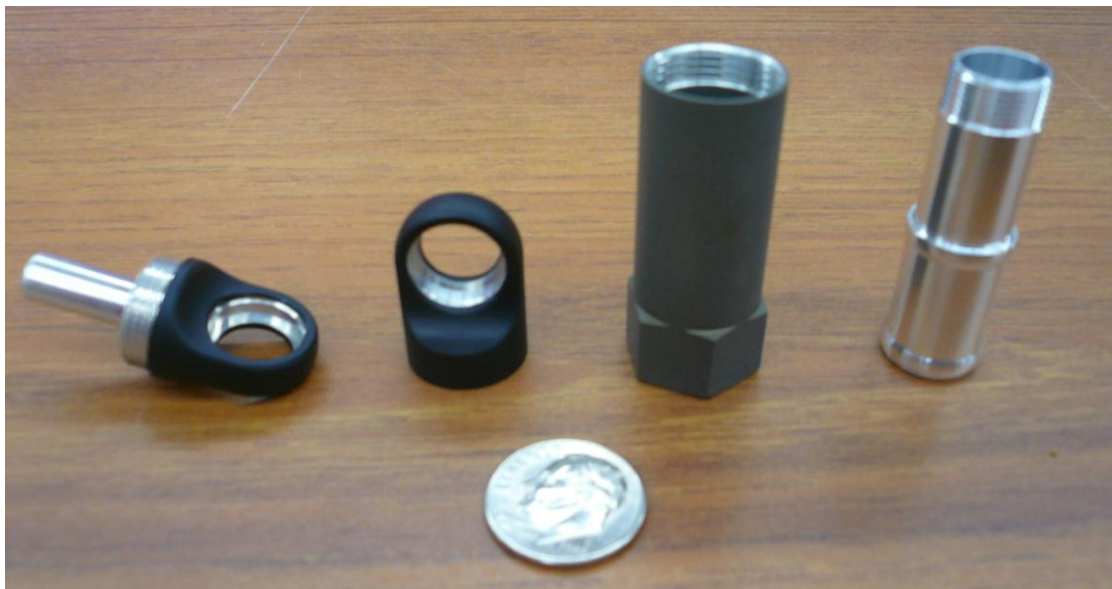
Figure 14 - Fabricated Strut Components
