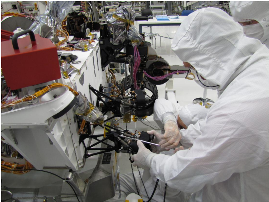
Figure 8 – Installation of BitBoxes onto MSL Rover
