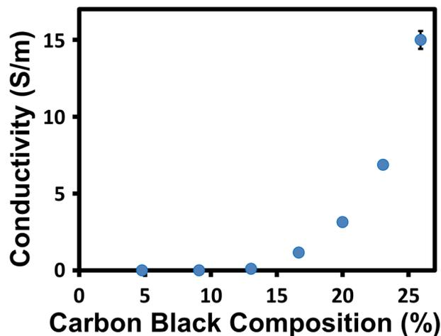
FIG. 2. Characterization of the carbon-PDMS electrodes. The conductivity of the carbon-PDMS composite material is measured with respect to the amount of carbon black material in the mixture.
