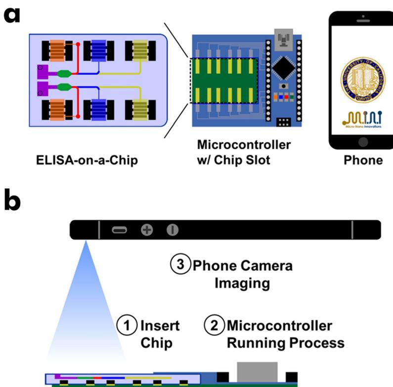
FIG. 1. (a) Integrated mobile-interfaced point-of-care system including a camera phone, an enclosed Arduino microcontroller on copper electrodes with a microfluidic chip slot, and a microfluidic ELISA-on-a-Chip. (b) Configuration with the microfluidic device inserted onto the copper electrodes and the phone camera imaging the ELISA reaction.
