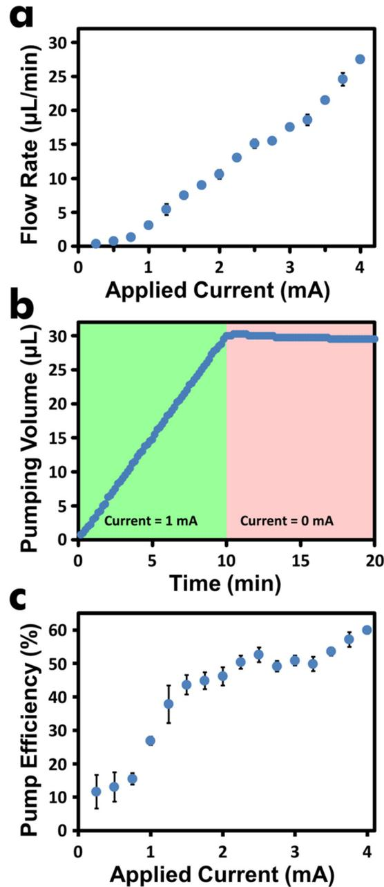
FIG. 3. (a) Characterization of the electrolytic micropump flow rate with the amount of current applied. (b) Electrolytic micropump is operated at 1 mA for 10 min with a steady increase in measured pumped volume. Current is off between 10 and 20 min time point. (c) Micropump efficiency is determined at applied current up to 4 mA.
