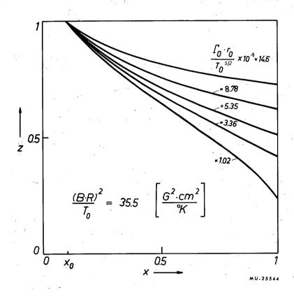
Fig. 3(a). Relative density distribution z(x) = n(x)/n for  $p_2 = 35.5$  and various parameter values of  $p_1$  [see Eq. (33)], calculated from Eqs. (28) and (29) for the example of cesium.
