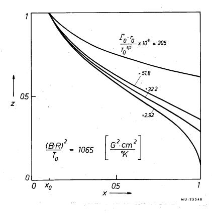
Fig. 5(a). Relative density distribution z(x) = n(x)/n for  $p_2 = 1065$  and various parameter values of  $p_1$  [see Eq. (33)], calculated from Eqs. (28) and (29) for the example of cesium.
