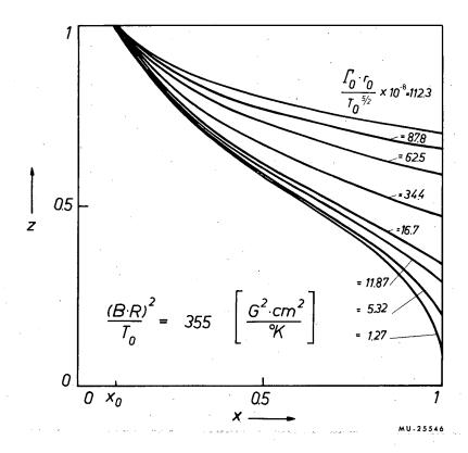
Fig. 4(a). Relative density distribution z(x) = n(x)/n for  $p_2 = 355$  and various parameter values of  $p_1$  [see Eq. (33)], calculated from Eqs. (28) and (29) for the example of cesium.
