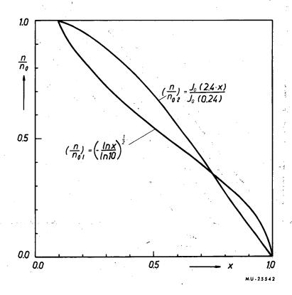
Fig. 1. Schottky approximation of the density distribution for the case of the fully ionized plasma column with external particle production  $\binom{n}{n_0}_1$ , and for the collision-dominated self-sustained positive column  $\binom{n}{n_0}_2$ .
