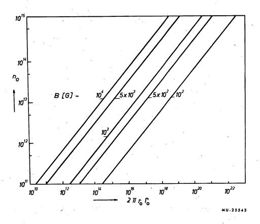
Fig. 2. Density  $n_0$  at the edge of the particle source calculated as a function of  $(2\pi\Gamma_0r_0/R)$  by using Schottky's approach.
