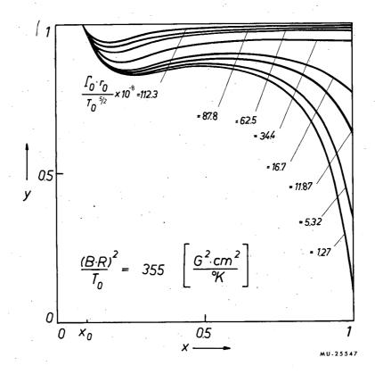
Fig. 4(b). Relative temperature distribution  $y(x) = T_{+}(x)/T_{0}$  for  $p_{2} = 355$  and various parameter values of  $p_{1}$  [see Eq. (33)], calculated from Eqs. (28) and (29) for the example of cesium.
