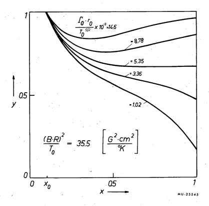
Fig. 3(b). Relative temperature distribution  $y(x) = T_{+}(x)/T_{0}$  for  $p_{2} = 35.5$  and various parameter values of  $p_{1}$  [see Eq. (33)], calculated from Eqs. (28) and (29) for the example of cesium.
