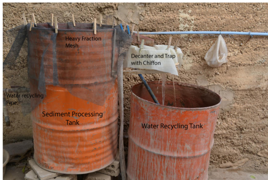
Figure 5.15: Modified Siraf-style flotation machine employed on the DEDP, with labeled component parts (Photo Martin Weber, 2012).
