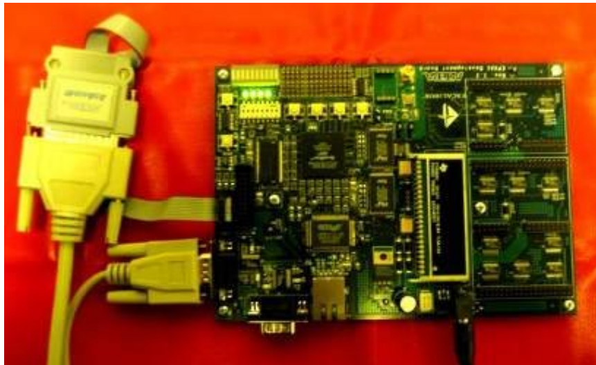
Figure IV.9: Experimental setup for demonstrating dynamic platform management using the Altera Excalibur development board
