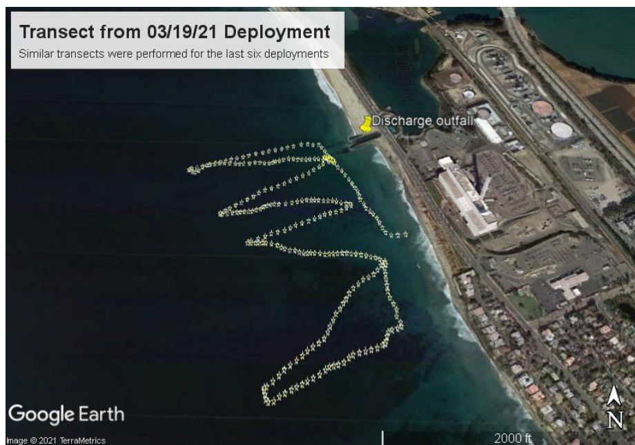
Figure 12 Two types of transects performed at the CDP study site. The first four deployments (top) collected data from north of the AHL inlet to south of the discharge outfall. The last six deployments (bottom) encompassed an area mostly south of the discharge outfall for higher data density (Google, 2021).
