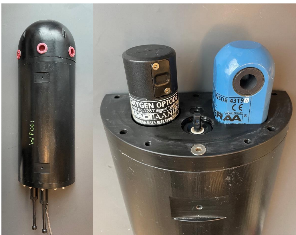
Figure 1 Preparing the WavepHOx for deployment on the stand-up paddle board (top). The fully assembled WavepHOx (left) and the sensor assembly under the end cap (right). From left to right, Aanderaa 3835 optode, Honeywell Durafet, and Aanderaa 4319 conductivity probe.
