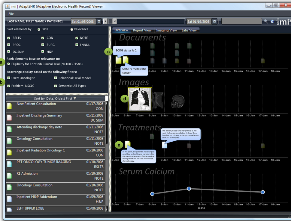
Figure 4.11: Screenshot of the AdaptEHR interface showing how the display is tailored to answer Query 8. (a) User specifies the context used to tailor the display. (b) The selected filters are used to instantiate the composition rules. (c) The display highlights concepts in documents that are relevant to the eligibility criteria. Phrases with terms that match variables in the model are extracted and presented to the user. All other documents are rendered transparently. (d) Related images are enlarged and highlighted. (e) Information regarding the patient’s past treatments is extracted and highlighted.
