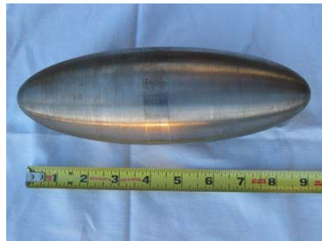
Figure 4.3.1: The 9 inch (23 cm) long and 3 inches (7.6 cm) in diameter steel ellipsoid.
