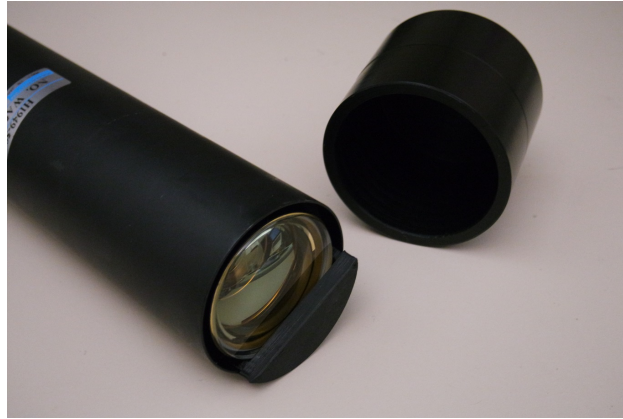
Figure 3.3: PMT with plastic positioning guard and external sleeve.
