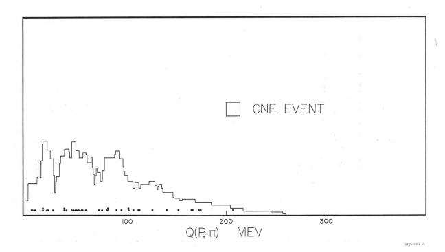
Fig. 7. Q(P,  $\pi$ ) distribution for protons and  $\pi^-$  from neutron stars in the propane.
