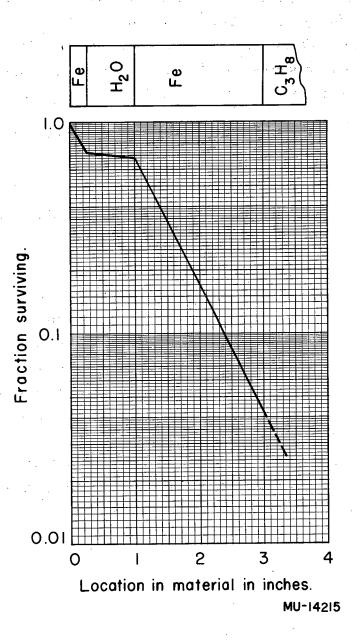
Fig. 15. Photon attenuation curve
