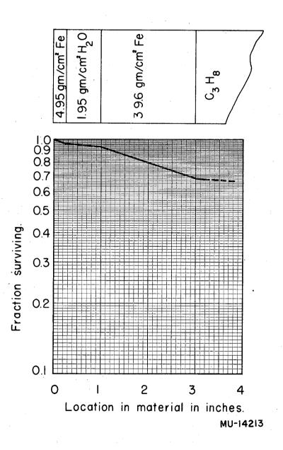
Fig. 12. Charged-particle attenuation curve.
