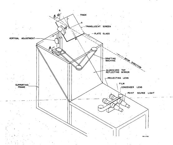
Fig. 5. Space-table schematic.
