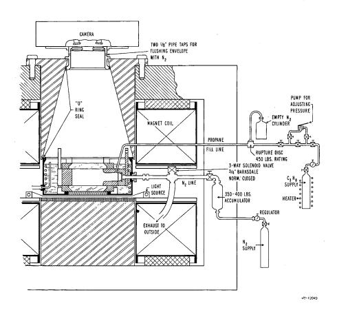
Fig. 3. Chamber in magnet.
