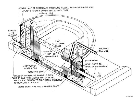
Fig. 2. Chamber assembly.
