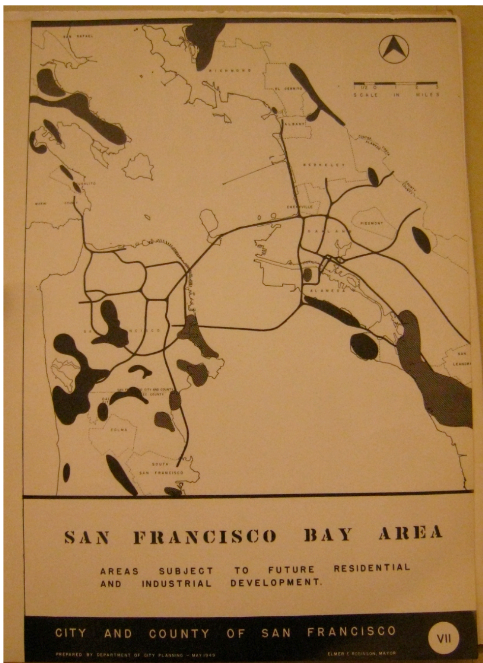
Figure 11: Map showing proposed southern crossing, and rail and highway lines from southern crossing, up eastern coast of San Francisco, into downtown. Grey indicates areas subject to future industrial growth; black indicates areas subject to residential development. Source: City and County of San Francisco, "The Case for the Southern Crossing," 1949, Box 2, Folder 1, Mayor Elmer Robinson Files, San Francisco History Center, San Francisco Public Library.
