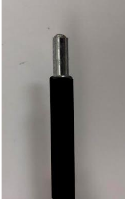
Figure 11: Cylindrical heat source used in ex vivo studies to mimic catheter ablation.
