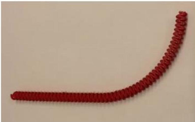
Figure 45: A 3D printed PLA support structure made of intersecting coils provide additional torsional stiffness for maneuverability after inserted.
