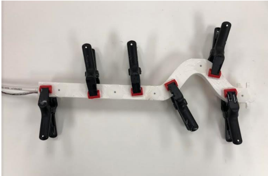
Figure 49: Clamped molds used during silicone curing process around the tubing with attached thermistors.
