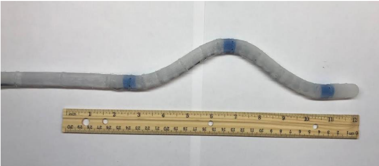
Figure 47: Prototype using thermoformed commercially available biocompatible tubing.
