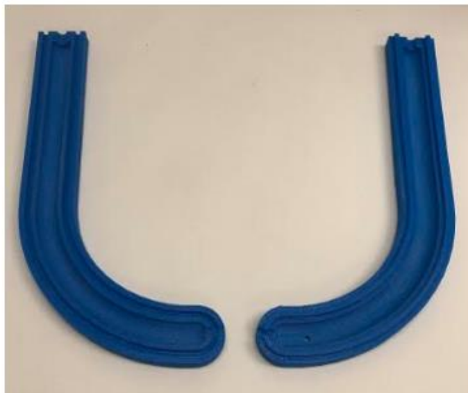
Figure 46: Two halves of the mold used to create the liquid silicone casting around the PLA support structure.
