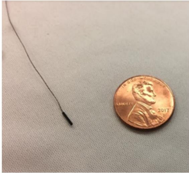
Figure 12: Commercially available 10 k \Omega NTC thermistors used in ex vivo studies.
