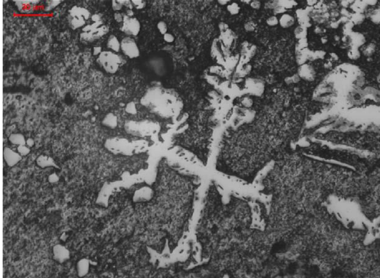
Figure 2.2: Precipitations in adherent PbLi scale [9].
