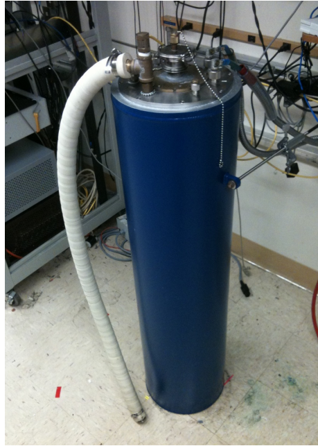
Figure 4.3: A photograph of the superconducting magnet system used in magnetotransport experiments in a custom designed liquid helium dewar.
