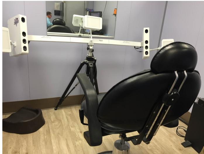
Figure 2. Adjustable chair with 3dMD photogrammetric system.
