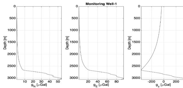
**Figure 5.** Examples of Kimberlina multiphysics data for training the DL single-physics and multiphysics networks. (a) Surface seismic modeling data. (b) Borehole-to-surface EM modeling data. (c) Surface and borehole gravity data.
